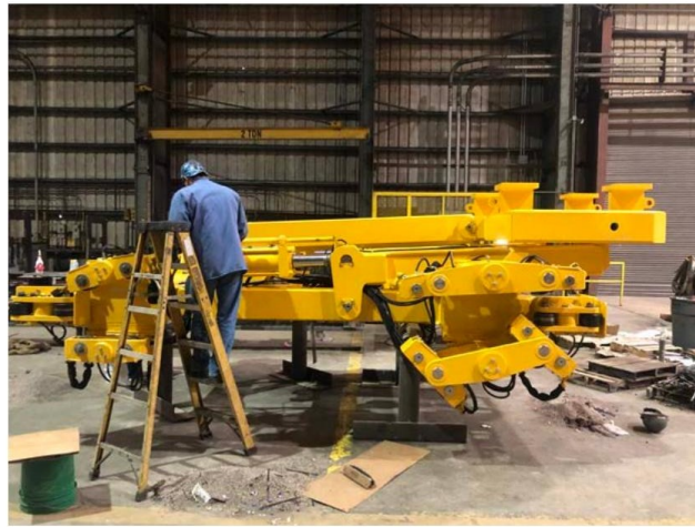
Figure 2 — Side elevation view showing hydraulic cylinder, arm linkage assembly, and lower arm connection points during final assembly verification
