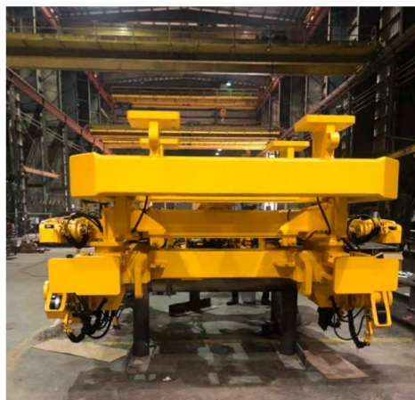
Figure 1 — Front view of the TDY-1250 Block Dolly following disassembly, inspection, structural repairs, and 3-coat marine paint application
